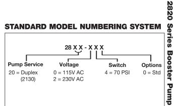
System The standard model numbering system is used for models up to -500. Numbers -500 and over are used for variations from standard assemblies such as special pump or tank specifications. Consult the factory for special models to meet specific requirements.
